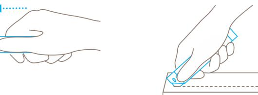
Use the slider to **engage the blade** for cutting.
