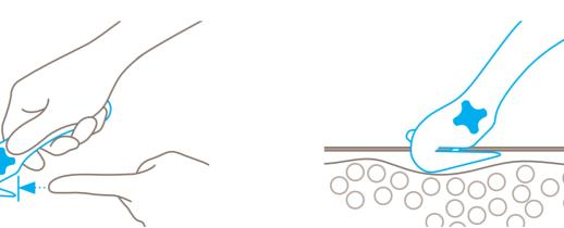
The concealed blade provides a maximum degree of **protection from cut injuries**.
